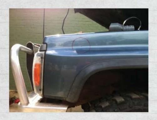
The 90 degree elbow that will sit in here will need to have an elongation in the hole to allow the inner radius of the 90 degree bend to sit inside too otherwise the snorkel wont sit close to the panel.
