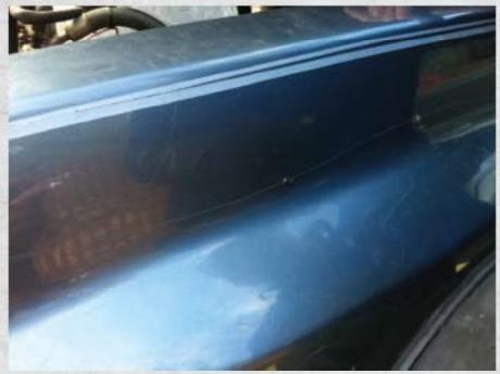
Time to mark out the circumferance of the rubber elbow that will go into the guard which can be tricky and you want to make sure It's correct... If unsure, start small and work your way out.
