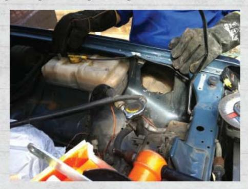
We now need to locate the centre of the hole to be cut on the outside guard. Use a punch or just anything sharp to punch the centre location from inside the engine bay. You don't need to punch it all the way through, just enough to locate the mark from the outer guard. The picture below is hard to see but you can just see a small punch mark to work off from the outside.
