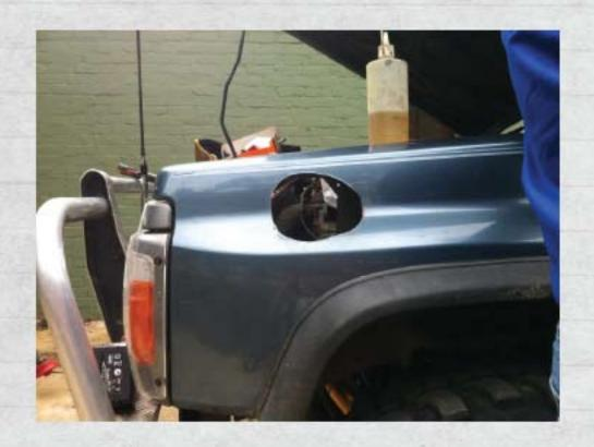
Prime, KillRust and or paint the cut. put the trim around the cut and silicone the outer trim to ensure no water can get in.
