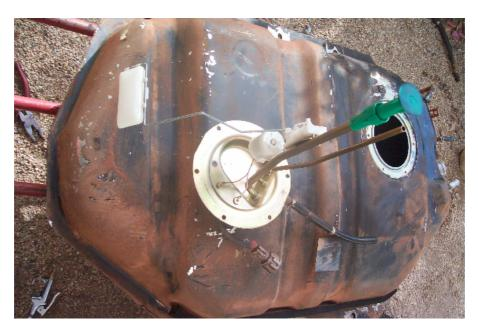
9. You can now drain and remove any slug etc from the tank...
