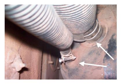
5. Unscrew the middle bolts holding up the fuel tank and slowly lower it down. The reason I say *SLOWLY*: there are the wires still connected on top off the tank.
