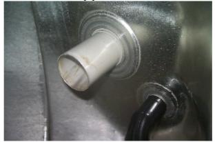
Where the fuel intake sits in – there's a 1cm ridge, which probably /obviously/maybe stops slug etc from messing up the fuel line intake
