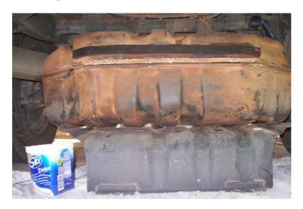
6. Disconnect the wires... be careful as these connectors are a pain to deal with... also a bit hard to disconnect off the tab on the tank
