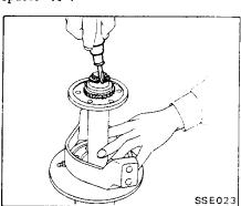
6. Remove spacer disc and bearing support.
