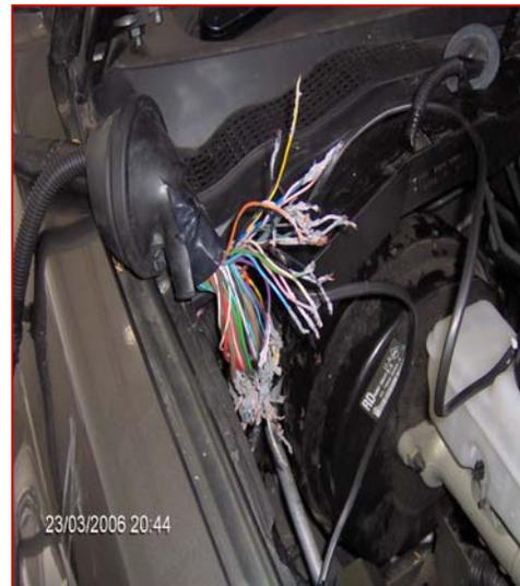
Main engine loom runs through the firewall to the right of the brake booster assy.
